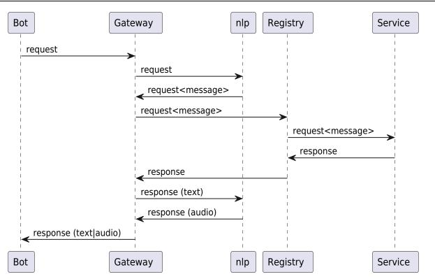
A user can write the *Bot* to request informations, the meaning of the message is extracted and a fitting *Microservice* is choosen to retrieve the necessary data. A response is build from that data and distributed back up to the bot which answers the users request.
