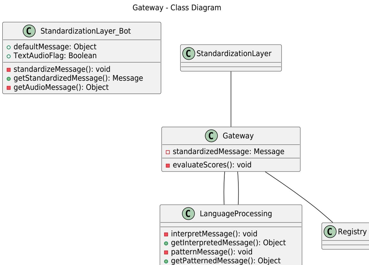
This class diagram shows the structure around the gateway. Here it is important that there is a StandardizationLayer beforehand, which standardizes the incoming messages. The gateway then directs the message to an NLU service where we get the evaluated object back and compare the scores. The best evaluated message is then forwarded to the registry.
